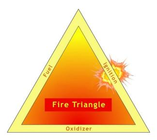
The storage and use of methacrylate esters have the potential for flammable vapors to develop. As indicated earlier, the polymerization inhibitors added to methacrylate esters require the presence of oxygen to function. Therefore, control of any fire risk from methacrylate esters generally focuses on the other two elements of the fire triangle, i.e., containment and control of ignition sources and avoiding creation of fuel (e.g., avoiding leaks and controlling vapors).
