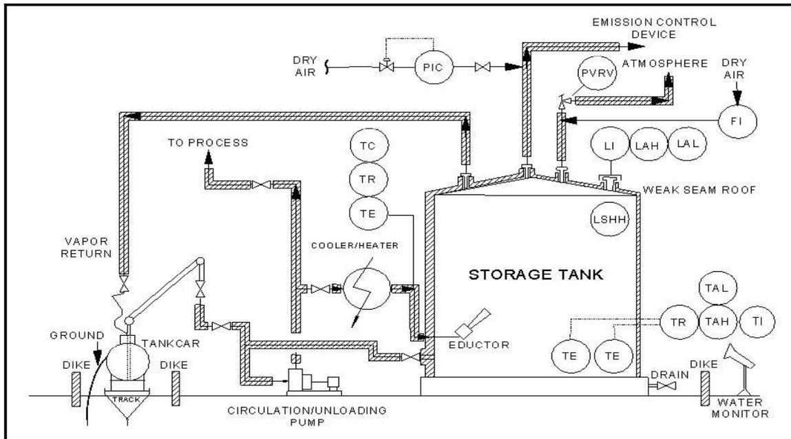
**Figure 12-1: Example of a Methacrylic Acid Storage Facility**
