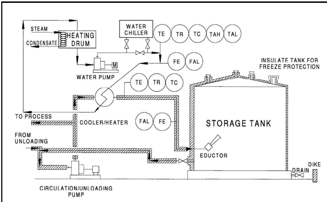
**Figure 12-2: Example of a Methacrylic Acid Storage Tank Temperature Control System**
