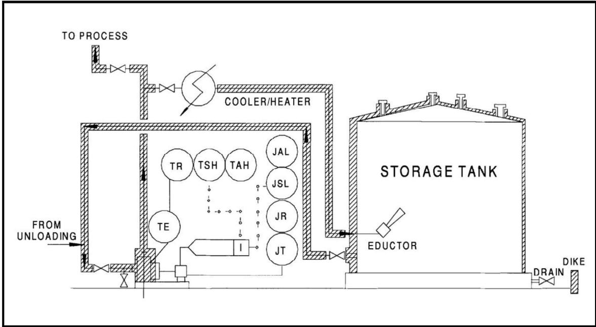
**Figure 12-3: Example of a Methacrylic Acid Pump Loop**
